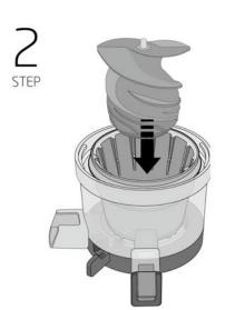
Press the squeezing screw into the assembled parts from [STEP 1] until the screw fits perfectly.
