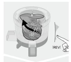
Press [REV] for 3-5 seconds to release pressure from chamber set. Repeat if necessary.
