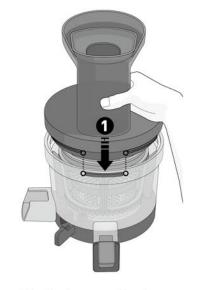
Place the assembled parts from [STEP 2] into the chamber by turning the strainer from side to side to fit the groove in the bottom bump of the chamber.
