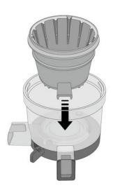
Assemble the chamber and ice cream strainer. Place the ice cream outlet align with juice outlet.
