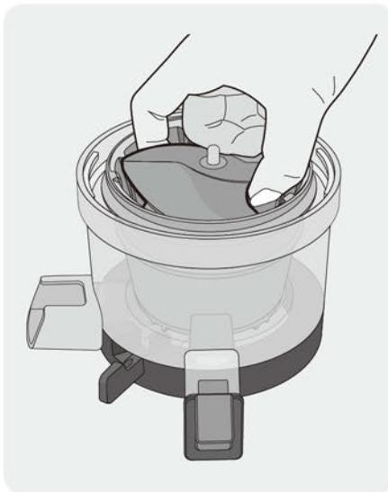
**3** Assemble the hopper like the picture. After putting the hopper on the chamber, turn it clockwise until it is locked completely.
