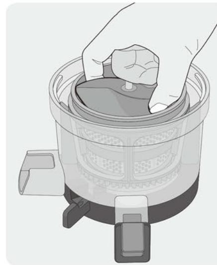
**4** Assemble the hopper like the picture. After putting the hopper on the chamber, turn it clockwise until it is locked completely.
