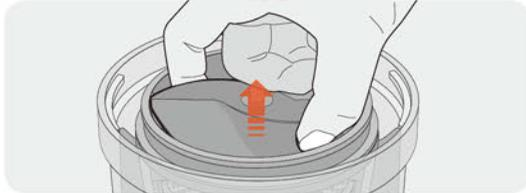
**3** Disassemble the strainer and spinning brush from the chamber.
