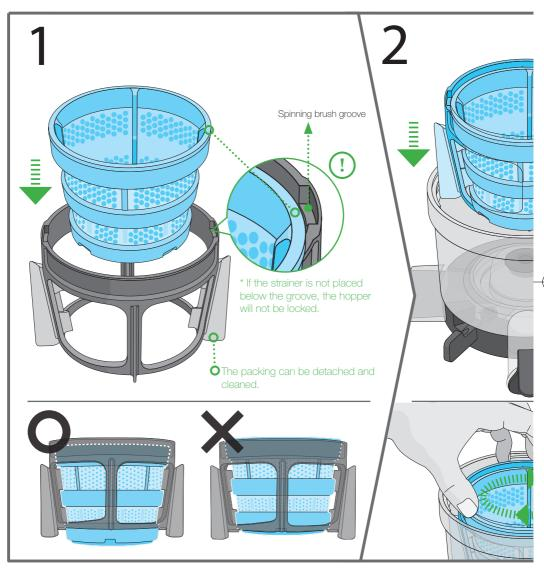
Assemble the strainer under the groove of spinning brush just like from the picture.
